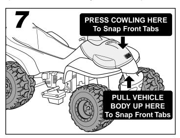
Press firmly on the front of the cowling to snap the four front tabs into the slots in the vehicle body. Make sure the side and rear tabs stay aligned with the slots.
